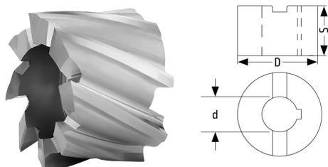
ISO 2586 DIN 1880 DIN 841  $\lambda 30^\circ$   $\gamma 12^\circ$
